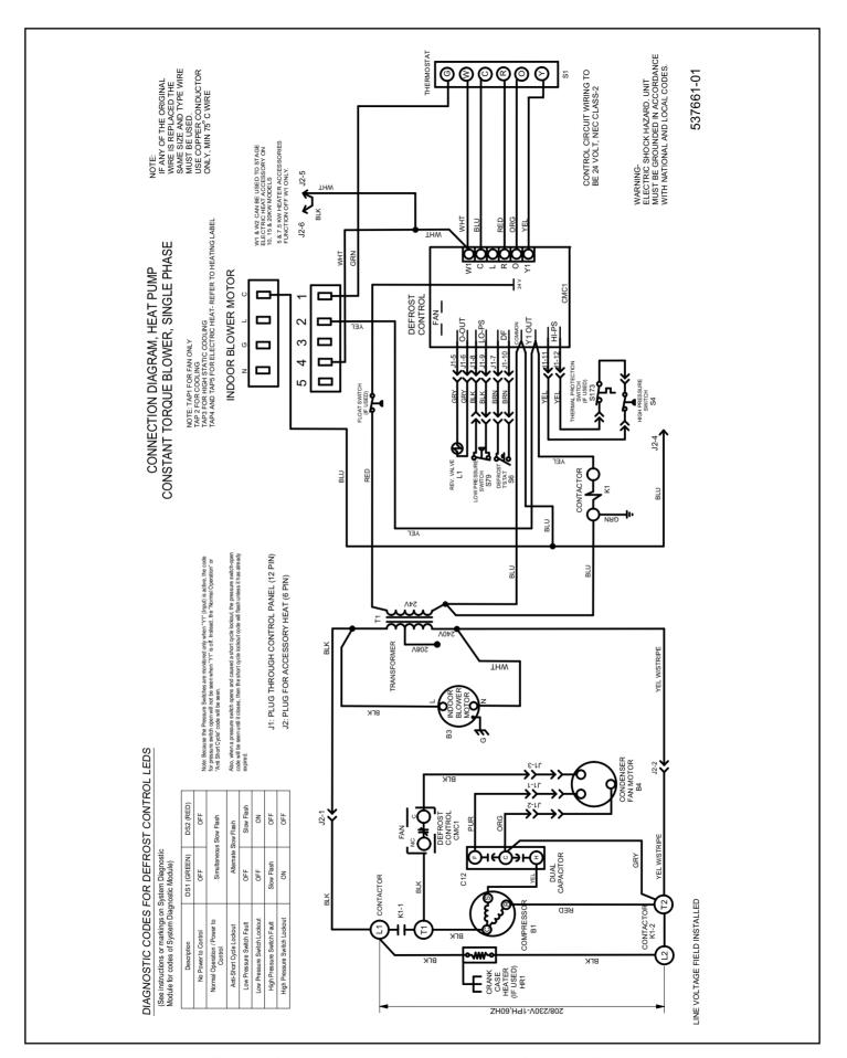
Figure 9. Connections Diagram - Heat Pump Constant Torque
