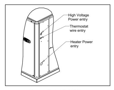
Figure 2. Typical Field Wiring
