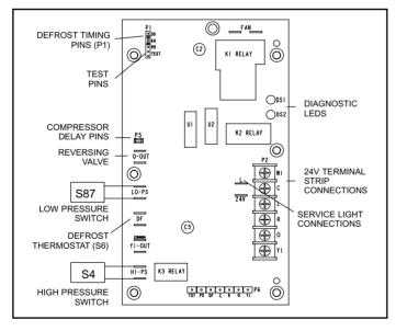
Figure 7. Defrost Control Board
