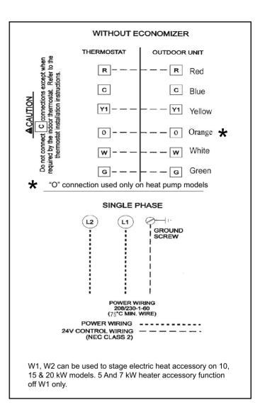
**Figure 4. Typical Wiring Connections**
