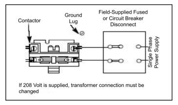
Figure 3. 208/230 Line Voltage Wiring
