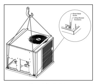
Figure 1. Rigging Unit
