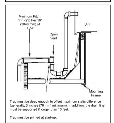
Figure 5. Typical Condensate Drain Connection
