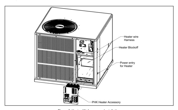
Figure 6. Heater Kit Accessory Installation
